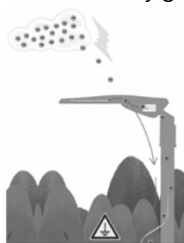
With effective grounding, the electric charge can be introduced to ground quickly
