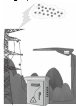
The SPD can absorb most surge energy before luminaire
